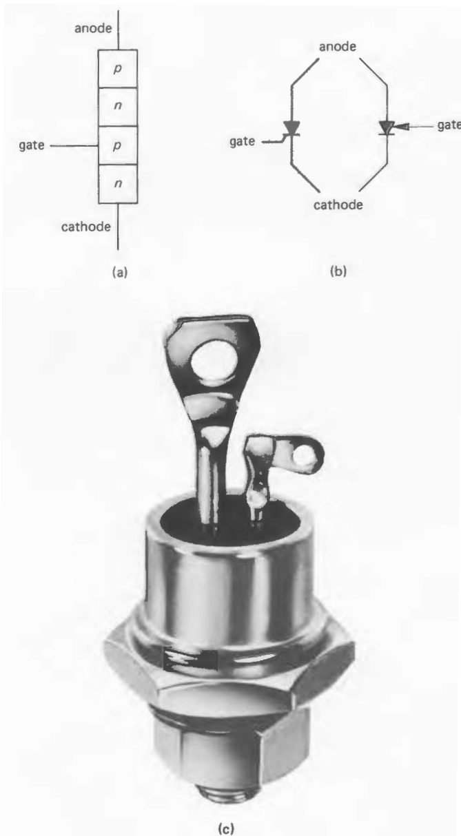
fig 16.10 (a) sectional diagram of a p-n-p-n reverse blocking thyristor, (b) circuit symbols and (c) a practical thyristor
