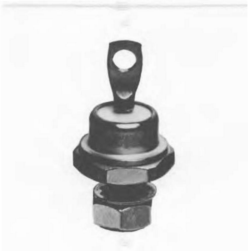
fig 16.2 photograph of (a) a signal diode and (b) a power diode
