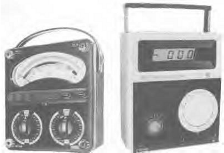
(a) an analogue multimeter, (b) a digital multimeter
